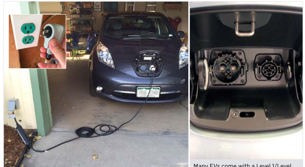
A “Level 1” cordset can be plugged in to a typical dedicated, 110-volt household outlet. Photos by Erik Nelsen, NREL 34794 (above) and 37587 (inset)
